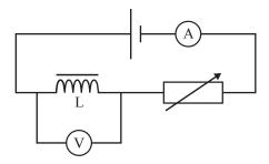
The resistance of the rheostat is changed so that the current in the circuit drops steadily from its maximum value of 1.62 A to 0.13 A in 1.2 s. While the current is dropping, the voltmeter reads 4.0 mV.
