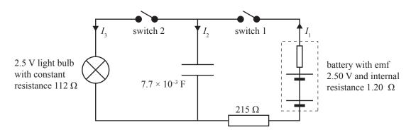
With switch 2 open, switch 1 is closed and the capacitor starts to charge.
