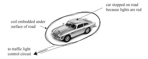
The inductance of the coil of wire must be measured. A possible way of doing this is to use a circuit like the one below. The inductor, L, in the circuit models the coil of wire under the road.
