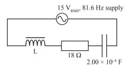
(c) In the space below draw and label phasors to show the voltages across the inductor, the capacitor and the resistor.
